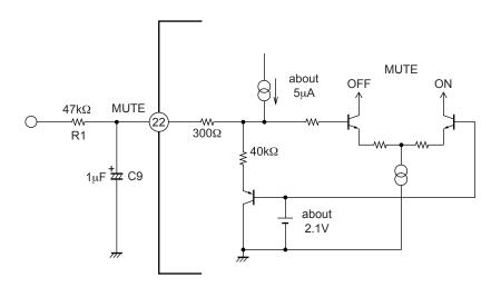
Fig2 Mute equivalent circuit
