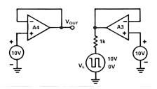
Figure 13a. Load Crosstalk Test Circuit
