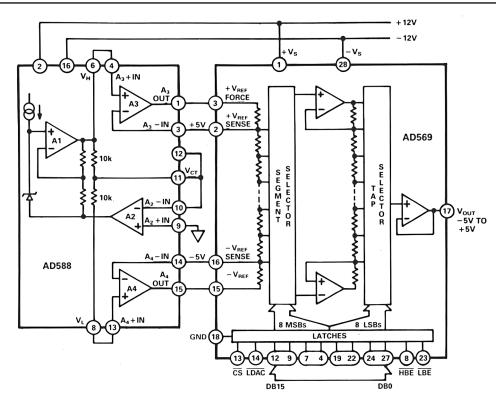
Figure 16. High Accuracy ±5 V Tracking Reference for AD569
