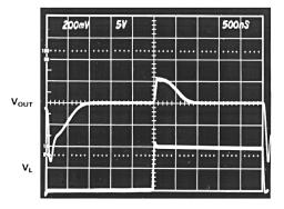
Figure 10b. Large-Scale Transient Response
