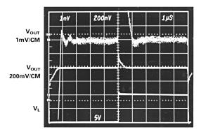
Figure 11b. Transient Response 5 mA-10 mA Load
