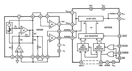
Figure 15. AD588/AD7535 Connections
