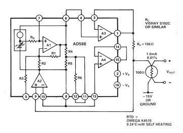
Figure 19. Precision Current Source for RTD
