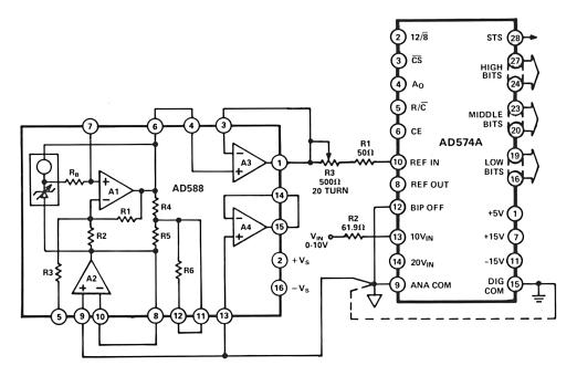
Figure 17. AD588/AD574A Connections
