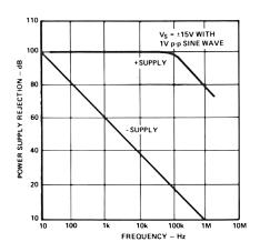
Power Supply Rejection vs. Frequency (A3, A4)
