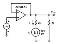
Figure 11a. Transient and Constant Load Test Circuit
