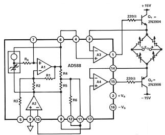
Figure 22. Bipolar Bridge Drive
