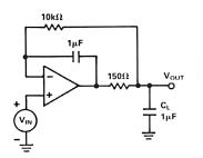
Figure 14b. Compensation for Capacitive Loads
