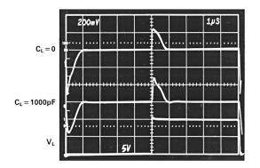
Figure 12b. Output Response with Capacitive Load
