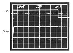
b. Extended Time Scale Figure 5. Turn-On Characteristics
