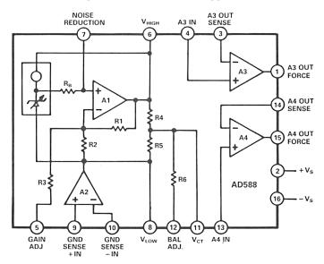
Figure 1. AD588 Functional Block Diagram
