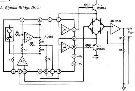
Figure 23. Floating Bipolar Bridge Drive with Minimum CMV
