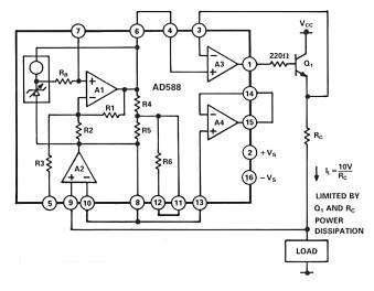
Figure 20. Boosted Precision Current Source
