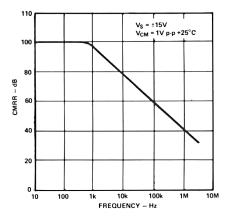
Common-Mode Rejection vs. Frequency (A3, A4)
