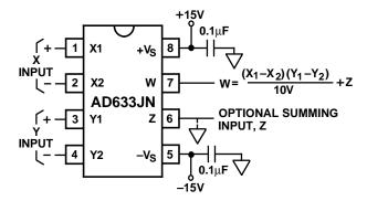
Figure 3. Basic Multiplier Connections
