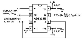
Figure 10. Linear Amplitude Modulator
