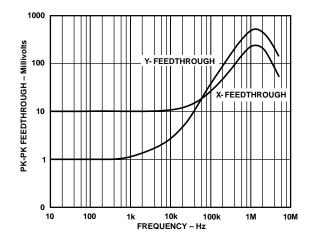
Figure 20. AC Feedthrough vs. Frequency
