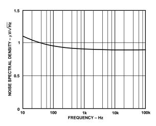
Figure 19. Noise Spectral Density vs. Frequency
