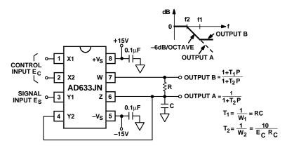
Figure 11. Voltage Controlled Low-Pass Filter
