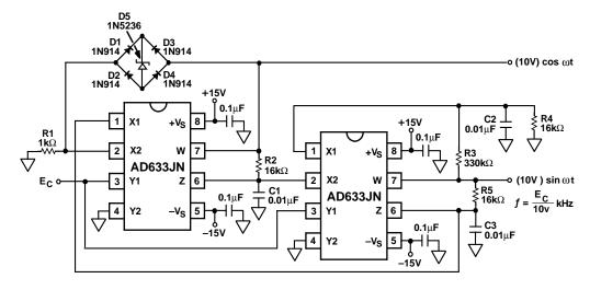
Figure 13. Voltage Controlled Quadrature Oscillator
