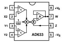
Figure 1. Functional Block Diagram (AD633JN Pinout Shown)
