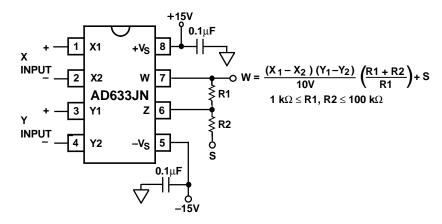
Figure 8. Connections for Variable Scale Factor
