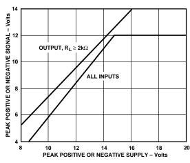
Figure 17. Input and Output Signal Ranges vs. Supply Voltages
