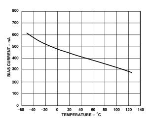
Figure 16. Input Bias Current vs. Temperature (X, Y, or Z Inputs)
