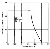
Figure 14. Large Signal Frequency Response
