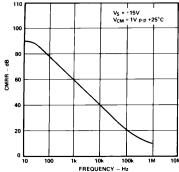
Figure 13. Common-Mode Rejection Ratio vs. Frequency
