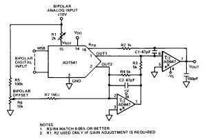
Figure 23. AD647 Used as DAC Output Amplifier
