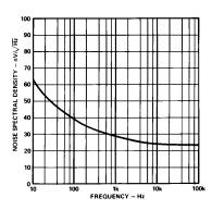
Figure 17. Input Noise Voltage Spectral Density
