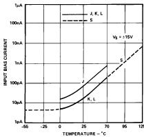
Figure 6. Input Bias Current vs. Temperature
