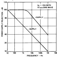
Figure 12. Power Supply Rejection vs. Frequency
