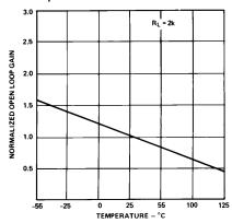
Figure 9. Open Loop Gain vs. Temperature
