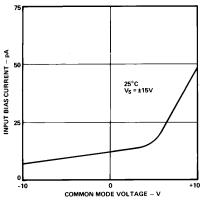
Figure 7. Input Bias Current vs. CMV
