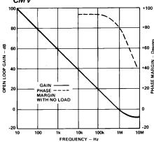
Figure 10. Open Loop Frequency Response
