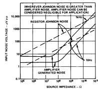
Figure 18. Total RMS Noise vs. Source Impedance
