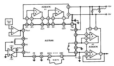
Figure 24. AD647 Used with AD7546 16-Bit DAC
