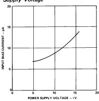
Figure 5. Input Bias Current vs. Power Supply Voltage
