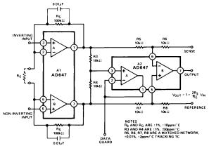
Figure 26. Precision FET Input Instrumentation Amplifier
