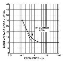
Figure 8. Input Noise Spectral Density
