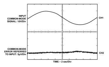
Figure 25. Instrumentation Amplifier Common-Mode Rejection
