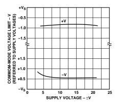
Figure 1. Input Common-Mode Range vs. Supply Voltage
