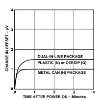
Figure 4. Offset Voltage Warm-Up Drift
