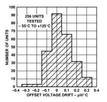
Figure 5. Typical Distribution of Offset Voltage Drift
