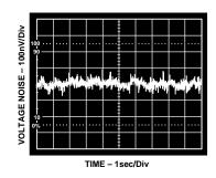
Figure 9. 0.1 Hz to 10 Hz Voltage Noise
