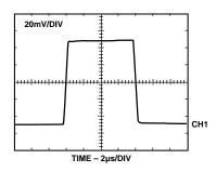
Figure 17. Small Signal Transient Response;  $A_V = +1$ ,  $R_L = 2 k\Omega$ ,  $C_L = 50 pF$
