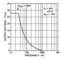
Figure 14. Large Signal Frequency Response
