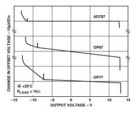
Figure 20. Gain Linearity of the AD707 vs. Other DC Precision Op Amps
