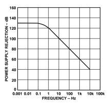
Figure 15. Power Supply Rejection vs. Frequency
