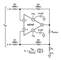
Figure 26. Precision Current Source/Sink
