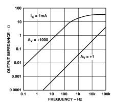
Figure 6. Output Impedance vs. Frequency
