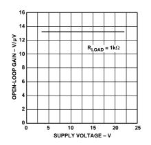
Figure 11. Open-Loop Gain vs. Supply Voltage
