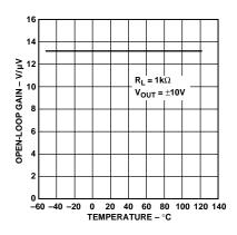
Figure 10. Open-Loop Gain vs. Temperature
