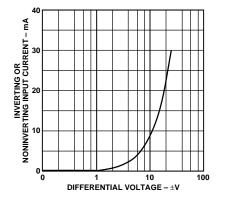
Figure 7. Input Current vs. Differential Input Voltage
