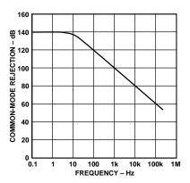
Figure 13. Common-Mode Rejection vs. Frequency
