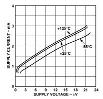
Figure 16. Supply Current vs. Supply Voltage
