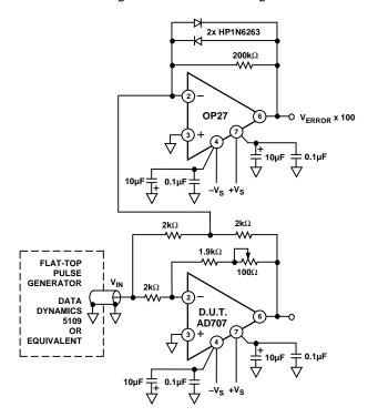
Figure 23. Op Amp Settling Time Test Circuit
