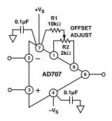
Figure 19. External Offset Nulling and Power Supply Bypassing
