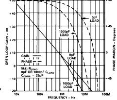
Figure 11. Open Loop Gain and Phase Margin vs. Frequency C<sub>COMP</sub> = 25 pF
