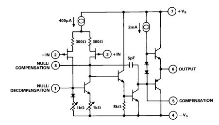
Figure 28. AD744 Simplified Schematic
