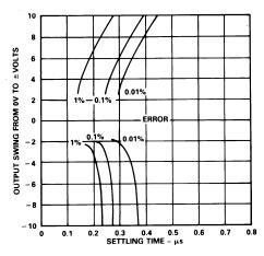
Figure 15. Output Swing and Error vs. Settling Time
