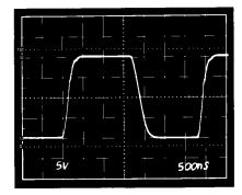
Figure 37. The Pulse Response of the 3 Op Amp Instrumentation Amplifier. Gain = 1, I Horizontal Scale:  $0.5 \mu V/div.$ , Vertical Scale: 5 V/div. (Gain= 10)
