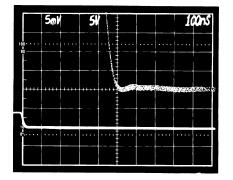
Figure 35. Upper Trace: AD744 Output Voltage for a +10 V to 0 V Step, Scale: 5 mV/div. Lower Trace: Logic Input Signal, Scale: 5 V/div.
