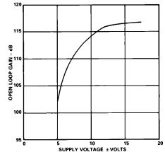
Figure 12. Open-Loop Gain vs. Supply Voltage
