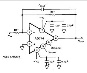
*Figure 32. AD744 Connected as an Inverting Amplifier Operating at Gains of 1 or Greater*
