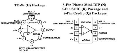
Alternatively, external decompensation may be used to increase the gain bandwidth of the AD744 to over 200 MHz at high gains. This makes the AD744 ideal for use as ac preamps in digital signal processing (DSP) front ends.
