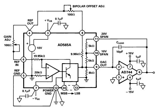
Figure 34. ±10 V Voltage Output Bipolar DAC Using the AD744 as an Output Buffer
