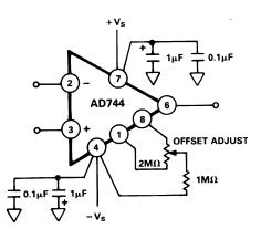
Figure 21. Offset Null Configuration
