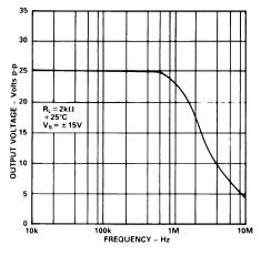
Figure 14. Large Signal Frequency Response
