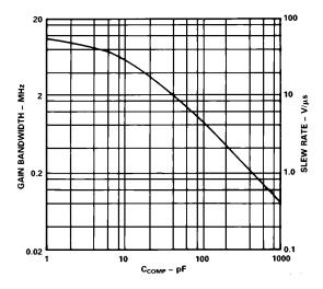
Figure 29. Gain Bandwidth and Slew Rate vs. C<sub>COMP</sub>
