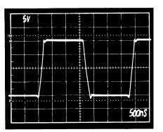
Figure 23b. Unity-Gain Inverter Large Signal Pulse Response,  $C_{COMP} = 5 \, pF$
