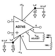
Figure 21. Offset Null Configuration, 8-Pin Package Pinout
