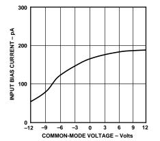
Figure 7. Input Bias Current vs. Common-Mode Voltage
