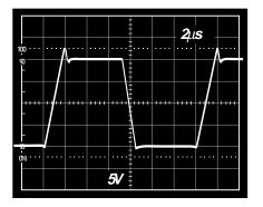
Figure 22b. Gain of 5 Follower Large Signal Pulse Response
