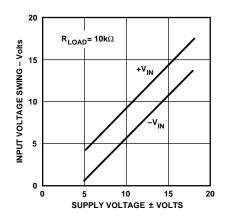
Figure 1. Input Voltage Swing vs. Supply Voltage
