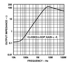
Figure 6. Output Impedance vs. Frequency
