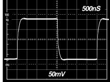
Figure 22c. Gain of 5 Follower Small Signal Pulse Response
