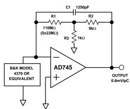
Figure 35a. A Basic Accelerometer Circuit
