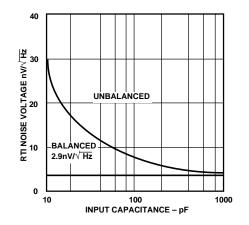
Figure 39. RTI Noise Voltage vs. Input Capacitance
