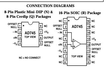
The AD745's guaranteed, tested maximum input voltage noise of 4 nV/ $\sqrt{Hz}$  at 10 kHz is unsurpassed for a FET-input monolithic op amp, as is its maximum 1.0  $\mu$ V p-p noise in a 0.1 Hz to 10 Hz bandwidth. The AD745 also has excellent dc performance with 250 pA maximum input bias current and 0.5 mV maximum offset voltage.
