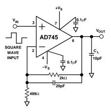
Figure 22a. Gain of 5 Follower, 8-Pin Package Pinout
