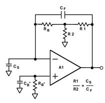
Figure 26. A Charge Amplifier Circuit
