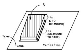
Figure 33. Breakdown of Various Package Thermal Resistance
