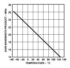
Figure 9. Gain Bandwidth Product vs. Temperature
