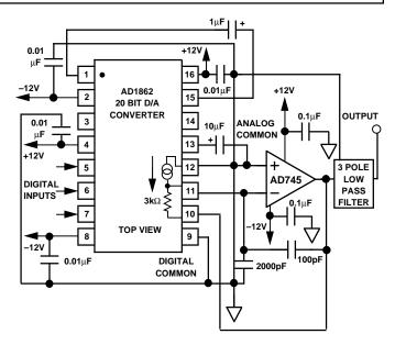
Figure 38. A High Performance Audio DAC Circuit
