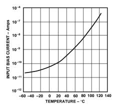
*Figure 5. Input Bias Current vs. Temperature*
