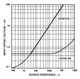
Figure 25. Input Offset Voltage vs. Source Resistance
