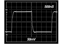
Figure 23c. Gain of 4 Inverter Small Signal Pulse Response
