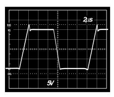
Figure 23b. Gain of 4 Inverter Large Signal Pulse Response
