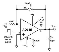
Figure 23a. Gain of 4 Inverter, 8-Pin Package Pinout
