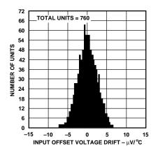
Figure 19. Distribution of Offset Voltage Drift.  $T_A = +25^{\circ}C$  to  $+125^{\circ}C$
