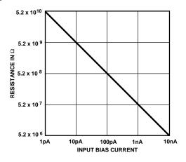
Figure 29. Graph of Resistance vs. Input Bias Current Where the Equivalent Noise  $\sqrt{4 \text{ kT/R}}$ , Equals the Noise of the Bias Current  $I_B(\sqrt{2qI_B})$
