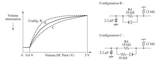
Fig. Volume characteristics of AN5270
