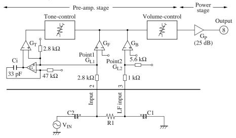
Fig. Simplified structure of AN5270 pre-amp. stage
