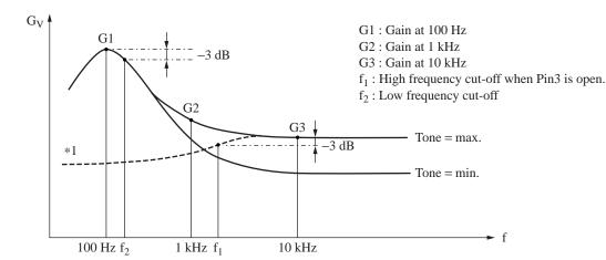
Fig. Frequency response of AN5270
