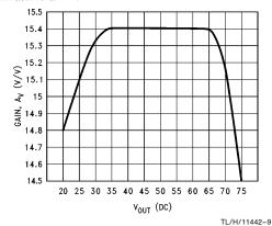
FIGURE 4. Gain vs  $V_{OUT}$  (DC),  $V_{IN} = 100 \text{ mV}_{PP}$
