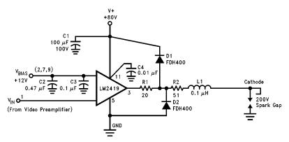
FIGURE 3. Typical Application Circuit (One Channel)
