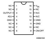
**Top View** Order Number LM2941WG/883 LM2941WG-QMLV. 5962-9166701QYA See NS Package Number WG16A
