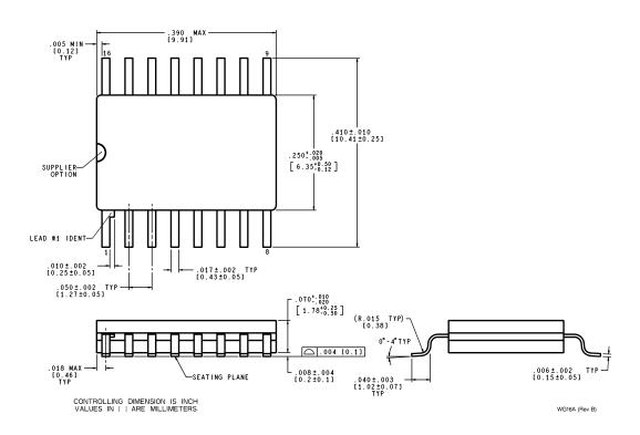
Order Number LM2941WG/883 LM2941WG-QMLV, 5962-9166701QYA **NS Package Number WG16A**
