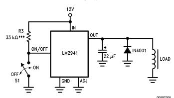
\*\*\* To assure shutdown, select Resistor R3 to guarantee at least 300 µA of pull-up current when S1 is open. (Assume 2V at the ON/OFF pin.)
