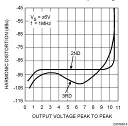
Harmonic Distortion vs. Output Voltage
