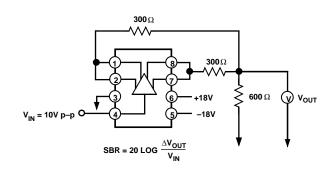
Figure 2. Signal Balance Ratio (BBC Method) Test Circuit
