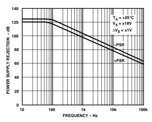
Figure 3. Power Supply Rejection vs. Frequency
