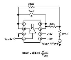
Figure 1. Output CMR Test Circuit
