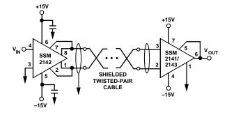
Figure 14. Typical Application of the SSM2142 and SSM2141
