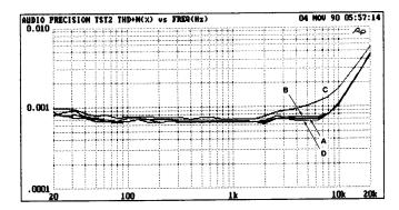
$V_{\rm O} = 10 \, {\rm V \ rms}$ , WITH 500 FEET CABLE
