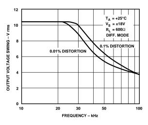
Figure 4. Maximum Output Voltage Swing vs. Frequency
