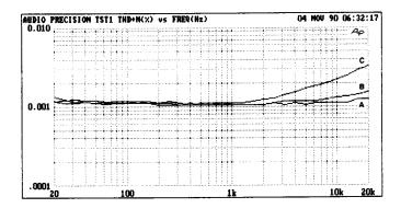
$V_{O} = 10 \text{ V rms}, \text{ NO CABLE}$  A: R1 = R2 = R<sub>L</sub> =  $\infty$  B: R1 = R2 = 600  $\Omega$ , R<sub>L</sub> =  $\infty$  C: R1 = R2 =  $\infty$ , R<sub>L</sub> = 600  $\Omega$
