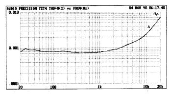
$V_{\rm O}$  = 10 V rms, NO CABLE A: R1 = R2 =  $\infty$ , R<sub>L</sub> = 600  $\Omega$
