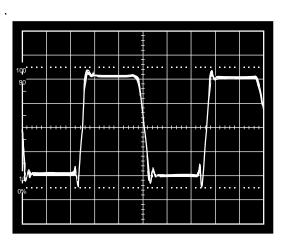
Figure 13. 100 kHz Square Wave at Point B (Differential Mode).  $V_O$  = 10 V rms, R1 = R2 =  $\infty$ ,  $R_L$  = 600  $\Omega$ , with Series Feedback Capacitors
