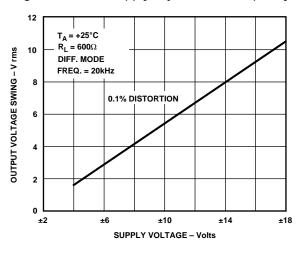
Figure 5. Output Voltage Swing vs. Supply Voltage
