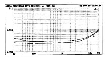
$V_O$  = 10 V rms, R2 = 0  $\Omega$ , R<sub>L</sub> =  $\infty$  A: R1 = 600  $\Omega$ , WITH 250 FEET CABLE B: R1 =  $\infty$ , NO CABLE
