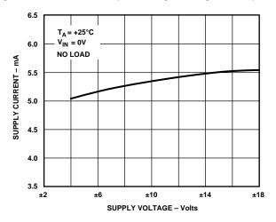
Figure 6. Supply Current vs. Supply Voltage
