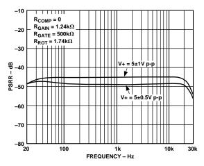
Figure 10c. PSRR vs. Frequency
