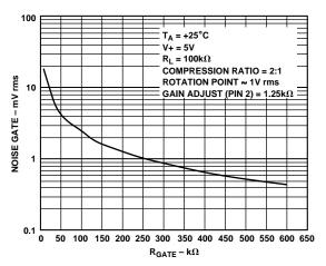
Figure 4. Noise Gate vs. R<sub>GATE</sub> (Pin 9 to V+)
