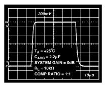
Figure 12. Large Signal Transient Response
