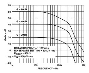
Figure 10b. GBW Curves vs. VCA Gain
