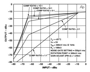
Figure 3. Output vs. Input Characteristics
