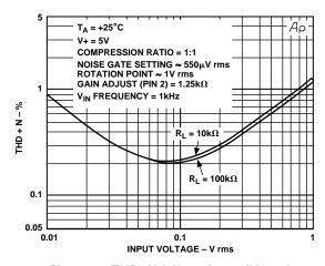
Figure 7. THD+N (%) vs. Input (V rms)
