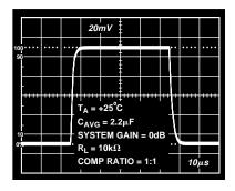
Figure 11. Small Signal Transient Response
