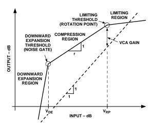
Figure 13. General Input/Output Characteristics of the SSM2166
