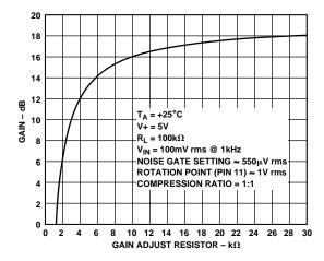
Figure 6. VCA Gain vs. R<sub>GAIN</sub> (Pin 2 to GND)
