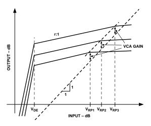
Figure 17. Effect of Varying the Rotation Point
