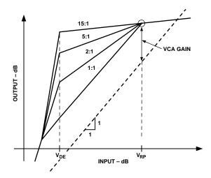
Figure 16. Effect of Varying the Compression Ratio
