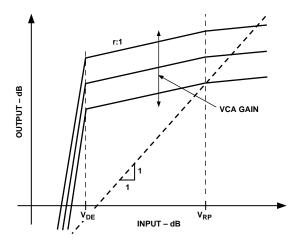
Figure 18. Effect of Varying the VCA Gain Setting
