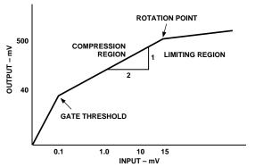
Figure 25. Transfer Characteristic
