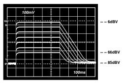
Figure 15a. RMS Level Detector Performance with  $C_{AVG} = 2.2 \, \mu F$
