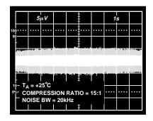
Figure 10a. Wideband Output Noise
