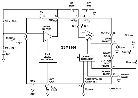
Figure 14. Functional Block Diagram and Typical Application
