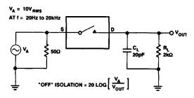
"OFF" Isolation Test Circuit
