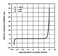
Leakage Current vs. Analog Voltage
