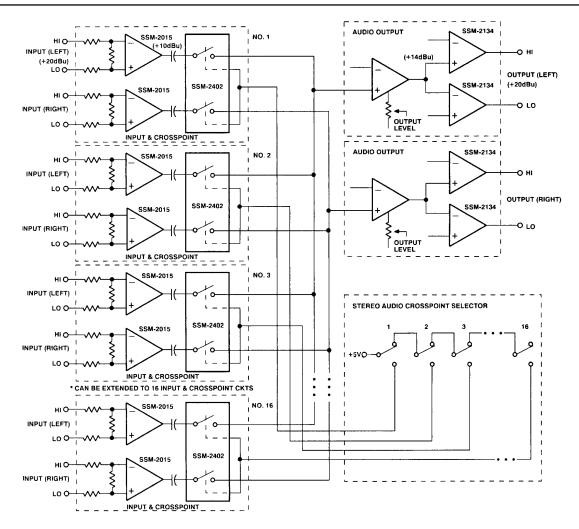
Figure 8. Switcher Functional Block Diagram
