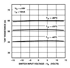
"ON" Resistance vs. Analog Voltage
