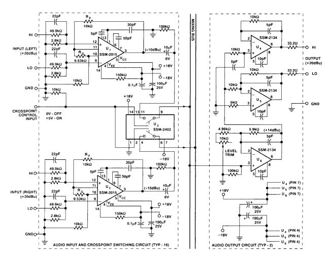
Figure 7. Switcher Schematic
