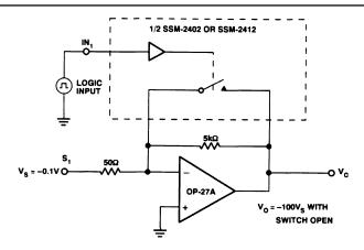
$T_{ON}/T_{OFF}$  Switching Response Test Circuit
