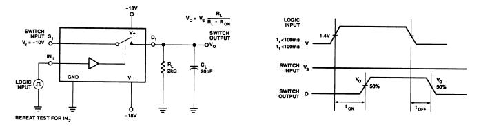
Switching Time Test Circuit
