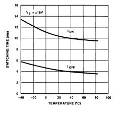
SSM2402 Switching Time vs. Temperature
