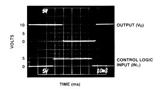
SSM2402 T<sub>ON</sub>/T<sub>OFF</sub> Switching Response
