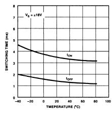
SSM2412 Switching Time vs. Temperature
