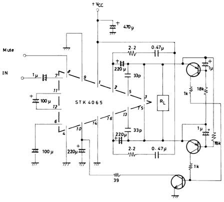
Sample Application Circuit of STK4065 Output Pin-to-V<sub>CC</sub> Short Protector
