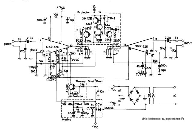
Sample Application Circuit (protection circuit and muting circuit)
