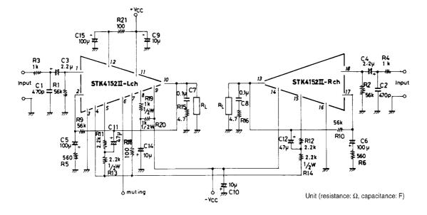
Sample Application Circuit: 30W min 2-channel AF power amplifier
