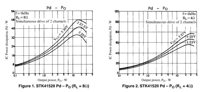
In an actual application where a music signal is used, it is impractical to estimate the power dissipation based on the continuous signal as shown above, because too large a heat sink must be used. It is reasonable to estimate the power dissipation as 1/10 Po max. (EIAJ).
