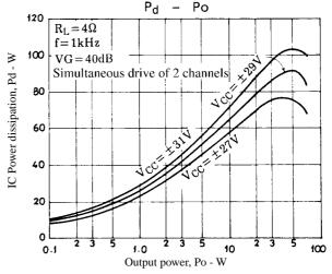
Figure 2. STK4172II Pd – Po ( $R_L = 4\Omega$ )
