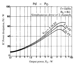
Figure 1. STK4182II Pd –  $P_O$  ( $R_L = 8\Omega$ )
