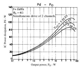
Figure 2. STK4182II Pd –  $P_0$  ( $R_L = 4\Omega$ )
