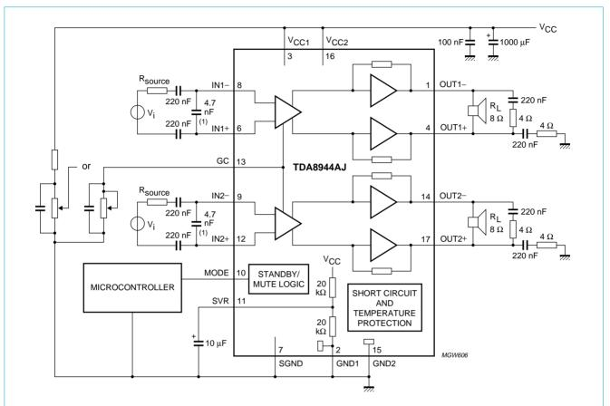
(1) To prevent high frequency oscillations do not leave the inputs open, connect a capacitor of 4.7 nF across the input pins close to the device.
