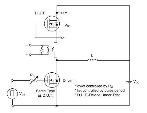
Peak Diode Recovery dv/dt Test Circuit
