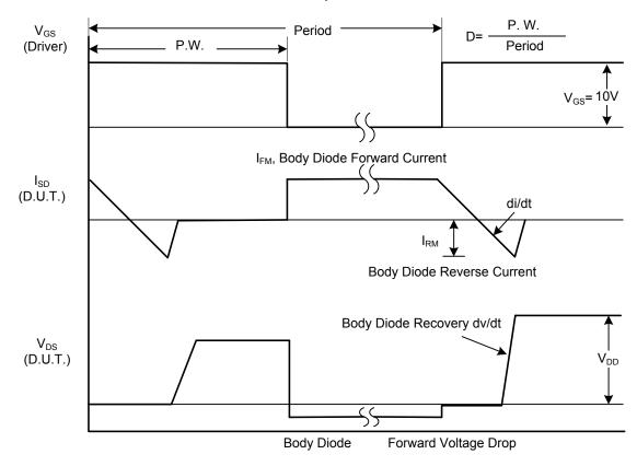
Peak Diode Recovery dv/dt Waveforms
