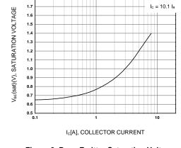
Figure 2. Base-Emitter Saturation Voltage
