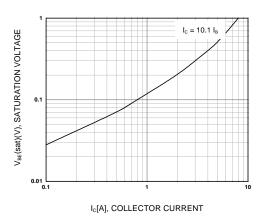
Figure 3. Collector-Emitter Saturation Voltage
