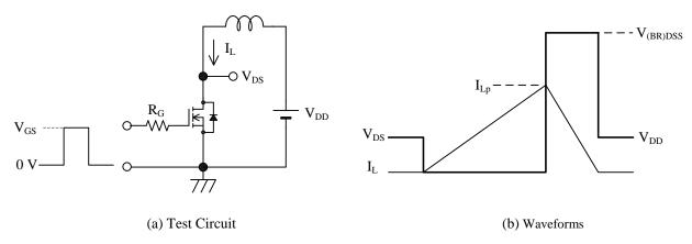
Figure 1 Unclamped Inductive
