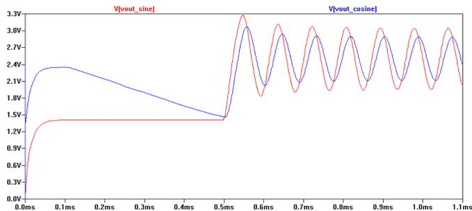
Note that oscillation does not occur while the current injection is taking place, but begins after the injection ends at 0.5ms. Some amplitude variance occurs before the circuit settles at its normal operational levels.
