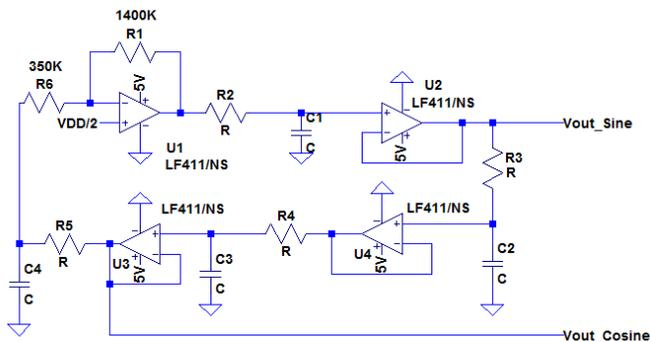
The resistors for the first inverting op-amp are selected to have a gain of four. Getting as close to this value as possible is desirable; gain slightly above four will cause the circuit to oscillate at a different frequency than desired, and gain less than four will not be high enough to sustain oscillation. While 1.4MΩ and 350KΩ were chosen, other values may be substituted. However, ensure that the resistor values used are large, as the
