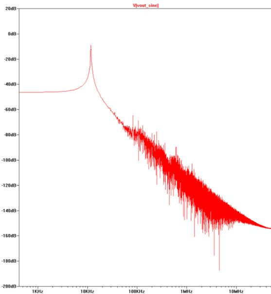
Once the FFT is performed, the THD can be calculated using Equation 2.
