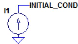
This current source is set up to inject a pulse of 20 mA for 0.4 milliseconds at the start of the simulation by using the PWL directive for the current source. This current injection is more than enough to get the simulation started; even briefer amounts of time would work. Equation 3 shows what the PWL specified by the simulation. The values alternate between times (0.0001, 0.0005) and the current output at those times (0.02, 0).
