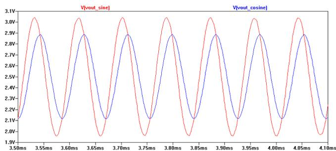
Two things should be noticed about the above plot: both waveforms have a DC offset of 2.5V, which is VDD/2. Also, the peak-to-peak value of the cosine wave is smaller than the peak-to-peak value of the sine wave. This is expected, and both the DC offset and peak-to-peak voltages can be altered by using additional filtering on the output lines.
