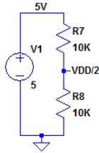
Using a voltage divider with equal valued resistors will provide the VDD/2 input to the circuit. Choose components in the 1KΩ-10KΩ range to reduce current flow through the voltage divider.
