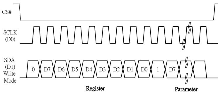
**Figure 6-3 : Write procedure in 3-wire SPI**
