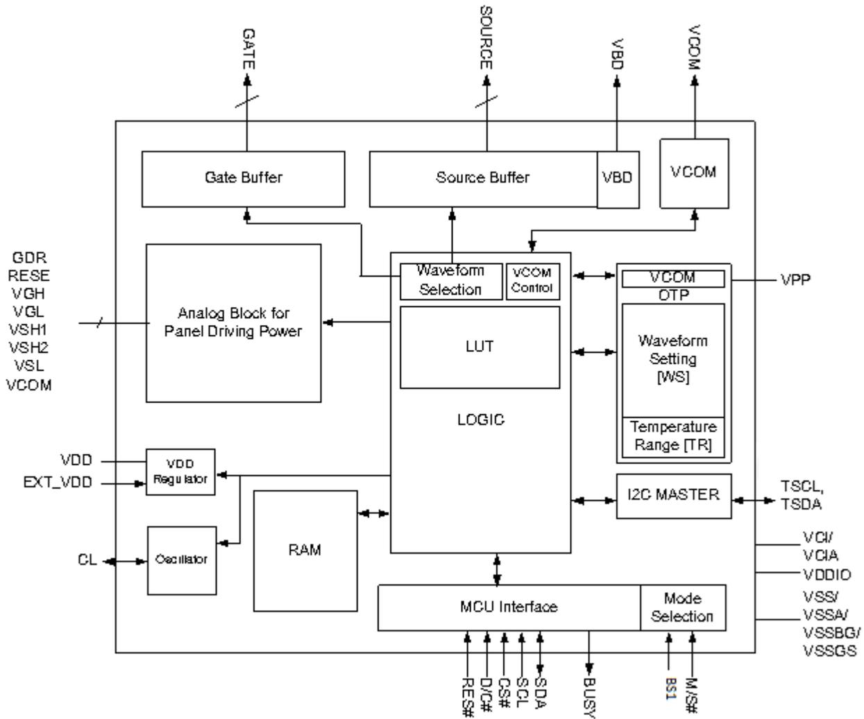
Figure 4-1 : SSD1675 Block Diagram
