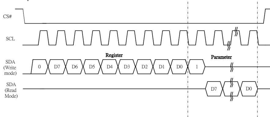
Figure 6-4 : Read procedure in 3-wire SPI mode
