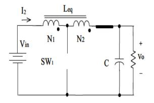
"When switch is "OFF": the diode is conducting and the magnetic element is being discharged through the equivalent inductance of  $L_1$  and  $L_2$ ."
