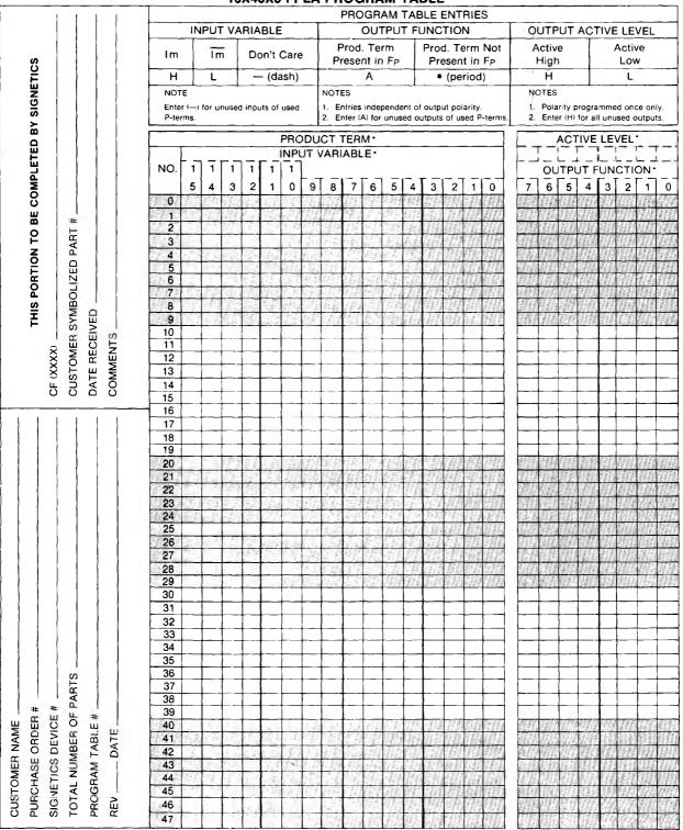
Input and Output fields of unused P-terms can be left blank. Unused inputs and outputs are FPLA terminals left floating
